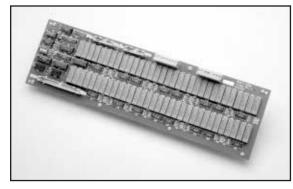
addressable MCPT-8X8 boards from a single METRABUS interface board. Additionally, any number of boards can be assigned the same board address, providing 2, 3 or N pole switches. Relay matrices can, therefore, be expanded in a linear (1 dimension), cartesian (2 dimensions) or geometric (3 dimensions) fashion creating versatile, multidimensional input and control schemes.
